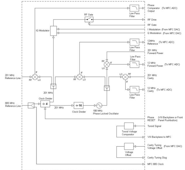
Figure 3: Block diagram of VXI RF module.
