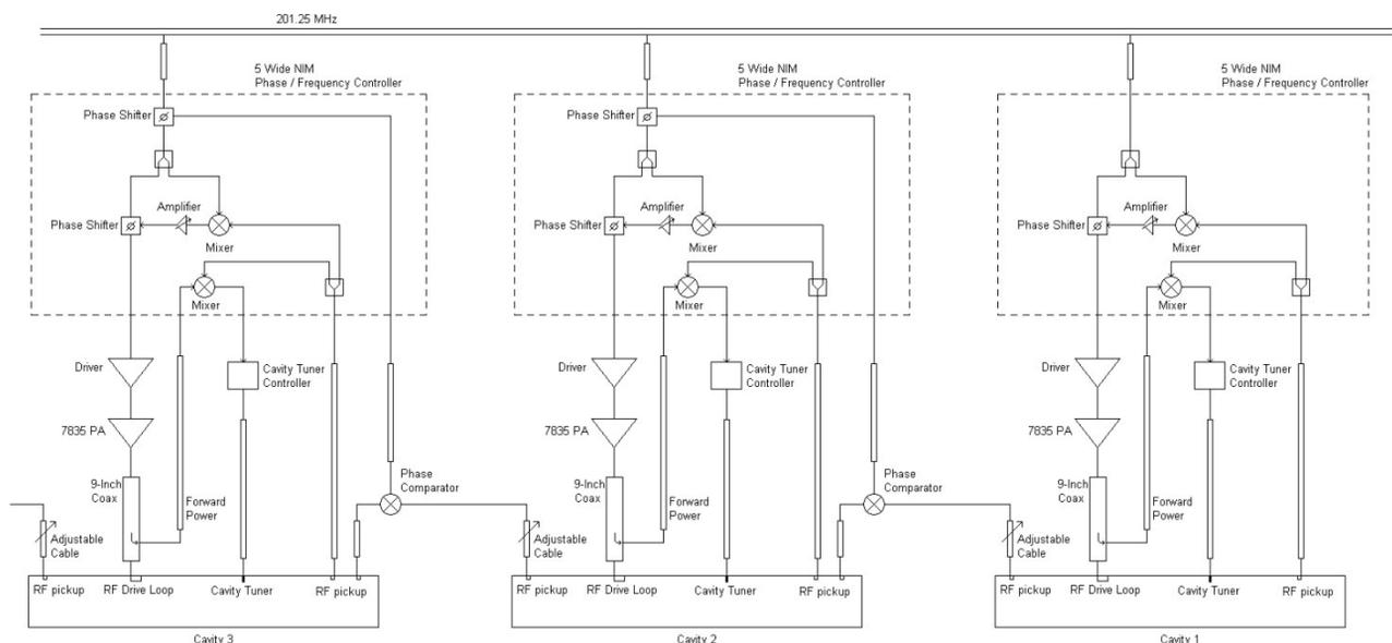
Figure 1: Simplified low energy (LE) linac RF block diagram of the present LLRF control system.
