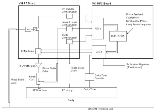
Figure 2: Block diagram of the new VXI LLRF system.
