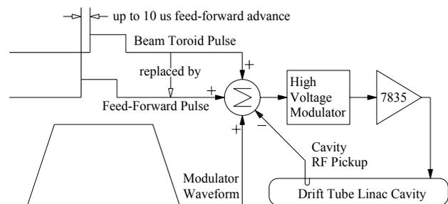
Figure 5: Modulator control system.
