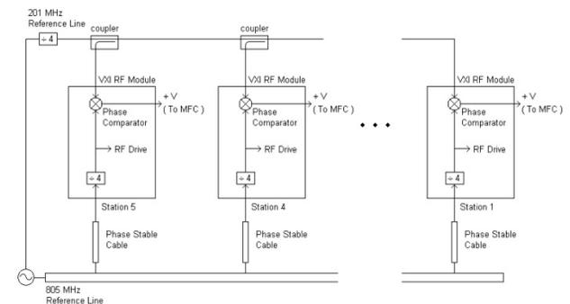
Figure 4: Block diagram of synchronous phase system.
