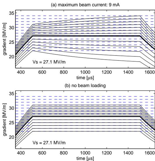
Figure 2: Amplitude plot for 13 cavities with (a) and without (b) beam.
