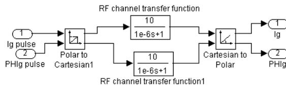
Figure 4: Block “RF channel”
