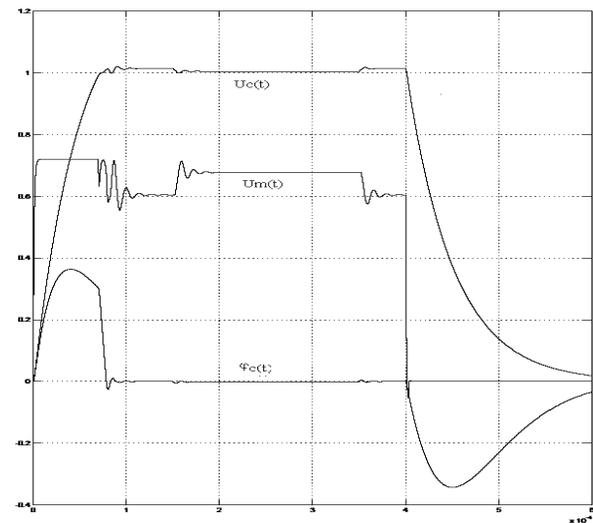
Figure 6: Envelope of RF voltage  $U_c(t)$ , phase  $\varphi_c(t)$  in the tank and anode modulator pulse  $U_m(t)$
