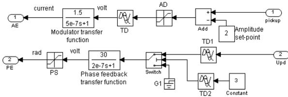
Figure 2: Model of the block "Feedback".
