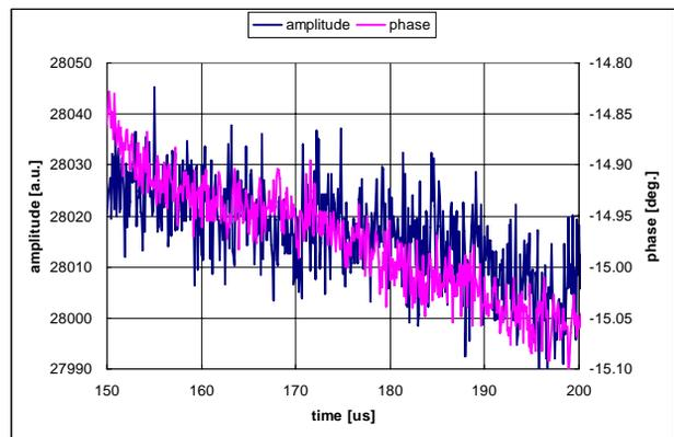
Figure 3: RF amplitude and phase in DTL cavity.
