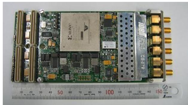
Figure 1: ICS-572B PMC Board.
