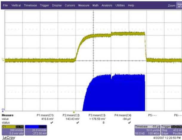
Figure 4(b): Feedback control with Feed-forward. (upper: Forward RF power, lower: Cavity field)
