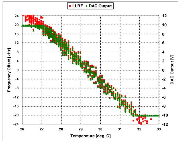
Figure 6: DAC output based on the measured frequency offset from the resonance.
