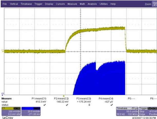
Figure 4(a): Cavity field response for feedback control. (upper: Forward RF power, lower: Cavity field)
