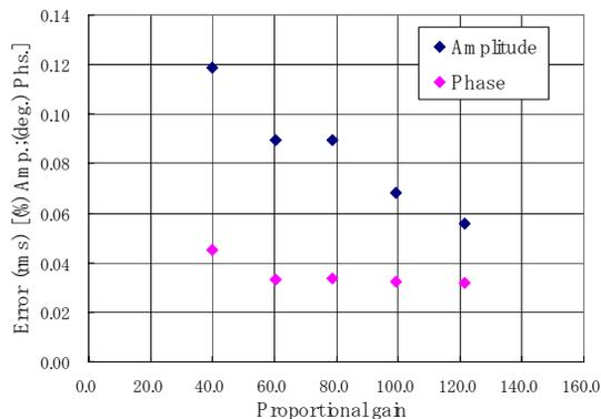
Figure 5: Errors in amplitude and phase at flat top.
