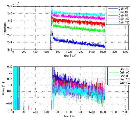
Figure 6: Amplitude and phase at the flat top with different proportional gain.
