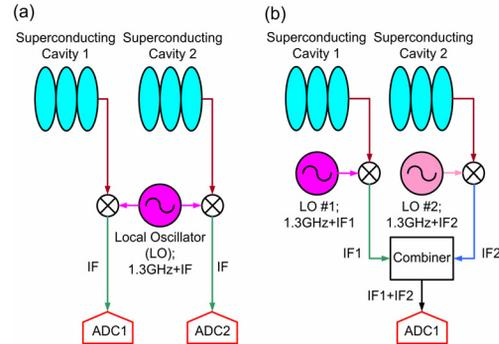
Figure 1: Schematic diagram of the digital LLRF system: a) conventional and (b) IF-mixture technique.
