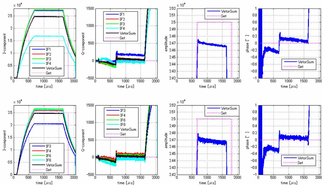
Figure 4: Measured I/Q and amplitude/phase components with FB operation for  $(M, N1, N2, N3, N4) = (9, 1, 2, 3, 4)$  and  $(24, 3, 4, 6, 8)$ .
