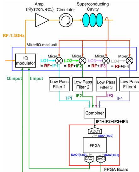
Figure 2: Schematic of system configuration.
