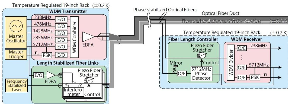
Figure 4: Schematic view of reference rf signals and the trigger-signal delivery system.
