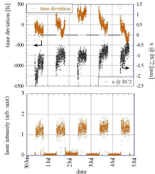
Figure 3: Trend of the arrival time (top), horizontal beam position measured at a dispersive section of the BC (middle) and the observed EUV laser intensity (down) for one week.
