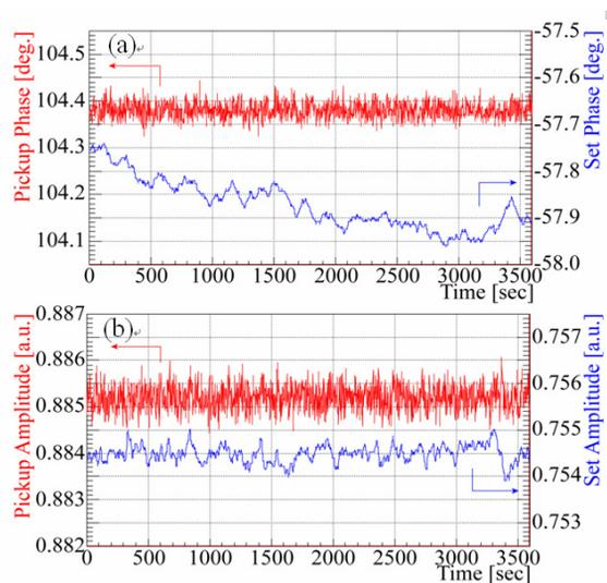
Figure 2: Set and measured value of (a) the phase and (b) the amplitude of the 238 MHz cavity pickup signal at the test accelerator.
