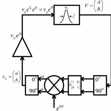
Figure 3: Basic I/Q driven mode with proportional feedback system.
