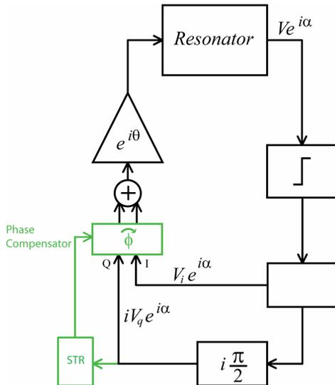
Figure 1: Phase-locked Self-excited loop with Self-Tuning phase compensator.
