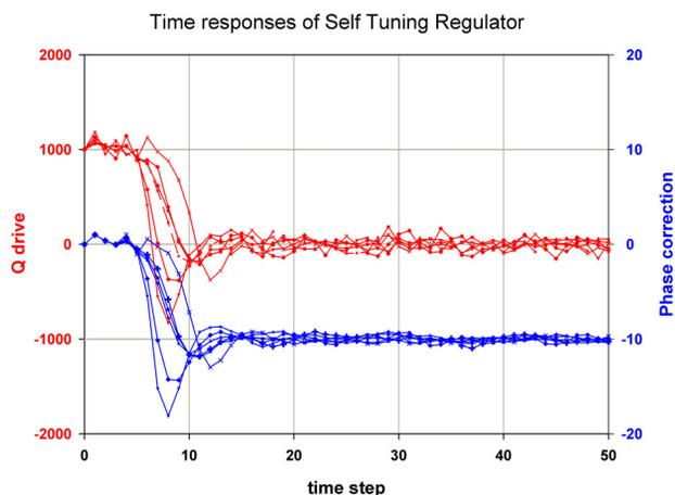
Figure 5: Simulation of Self Tuning Regulator for misalignment compensation.
