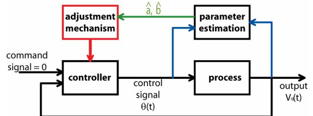
Figure 3: Block diagram of a self-tuning regulator.
