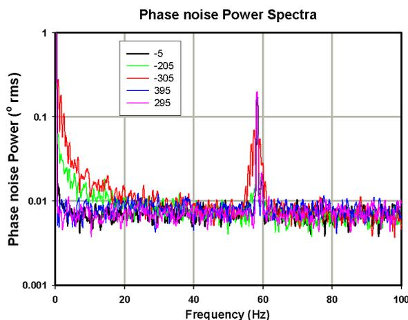
Figure 4: Phase noise of ISAC 2 cavity at different degrees of misalignment.
