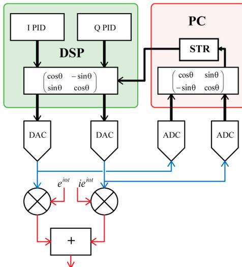
Figure 2: Implementation of phase rotator.
