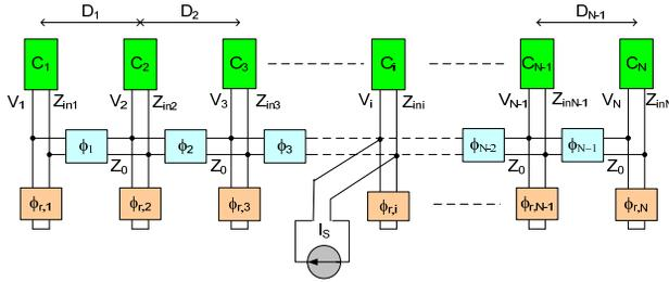
Figure 2 – A fan-out power distribution system in Figure 1(b) realized using phase shifts in transmission line phase delays and reactive loadings
