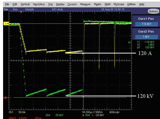
Figure 5: Arc-down test of Marx during full voltage operation, Ch1 is load current and Ch4 is load voltage.
