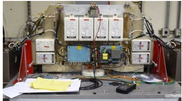
Figure 2: Photograph of one SNS H-bridge card on the SLAC single phase test stand.
