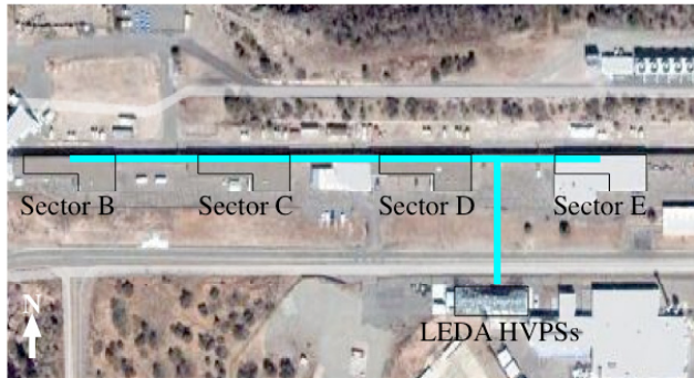
Figure 3: HV cable routing from LEDA power supplies to LANSCE capacitor rooms.[4]
