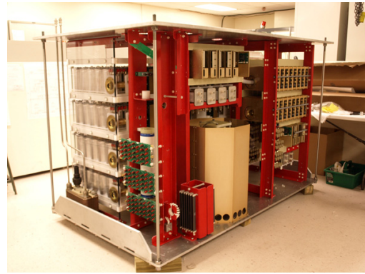
Figure 5: The ILC Modulator is presently being assembled into a compact unit, for immersion in a 7' x 5.5' oil tank, with controls on top and coax cable pulse output.
