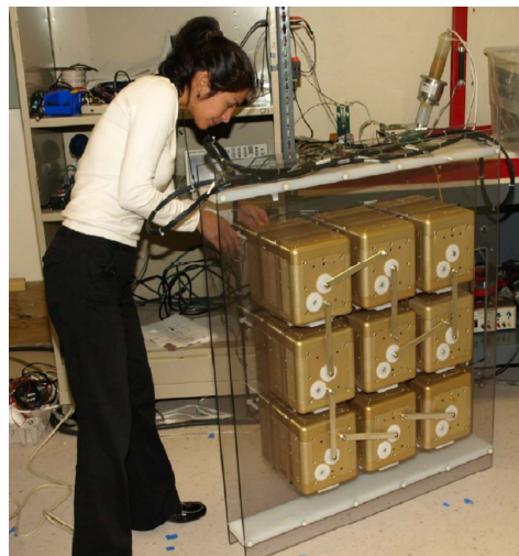
Figure 3: Nine cells of the short-pulse Marx mounted in a rack for system testing.
