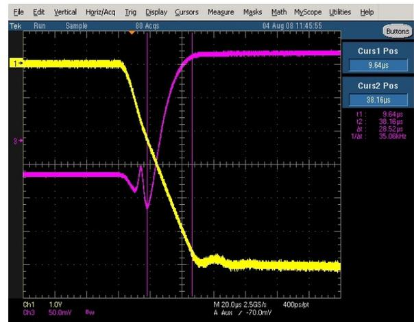
Figure 3: Time response of the 75 kW phase shifter biasing solenoid current (CH1 @ 50A/div.) and reflected phase (CH3 @ ~30 deg./div.) to a fast step (risetime < 1 µs) in the current program. The time scale is 20µs/div.
