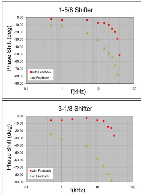
Figure 4: Phase shifter frequency responses with and without feedback.
