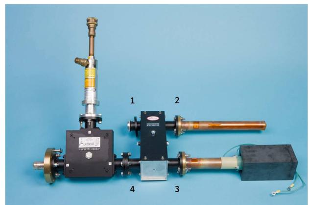
Figure1: Photograph of a 75 kW vector modulator.
