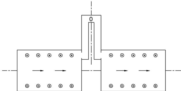
Figure 5: Quarter-wave-stub resonant coupler.
