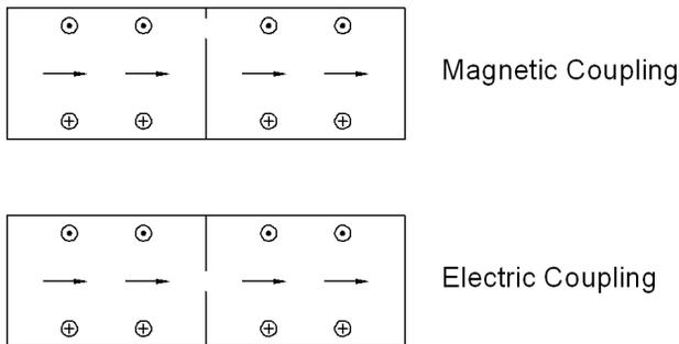
Figure 2: Examples of magnetic and electrical coupling.
