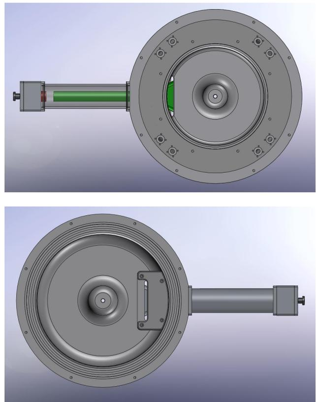
Figure 7: Two views of the resonant coupler.
