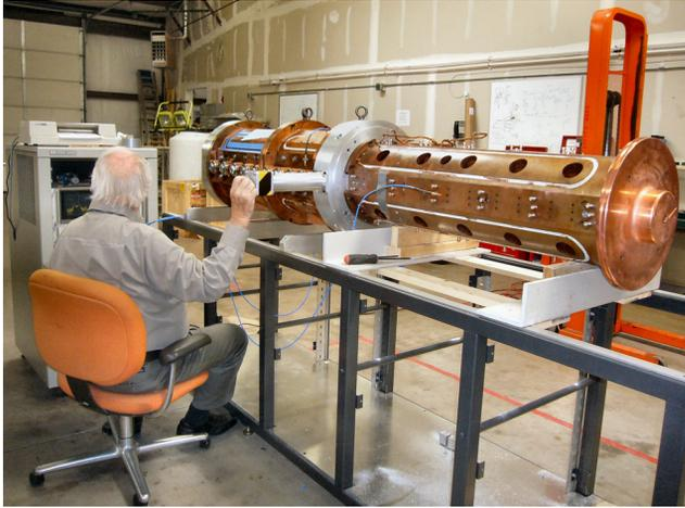
Figure 6: A 1.1-MeV RFQ linac resonantly coupled to a 3.5-MeV RFI linac with a quarter-wave-stub resonant coupler.
