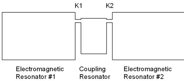
Figure 1: Diagram of resonantly coupled resonators.
