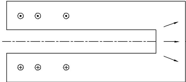
Figure 4: Generic quarter-wave stub resonator.
