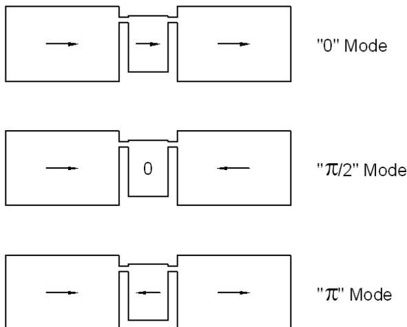
Figure 3: Basic modes of three coupled resonators.
