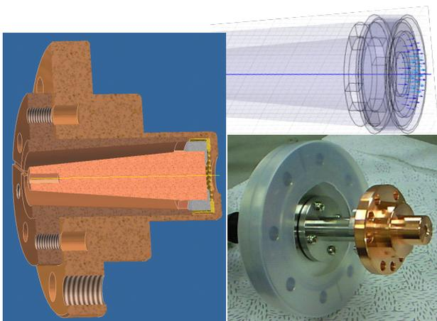
Figure 2: The C-band input cavity of the test tube.
