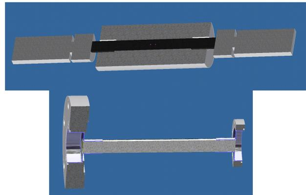
Figure 4: The X-band dielectric waveguide for the insulation.
