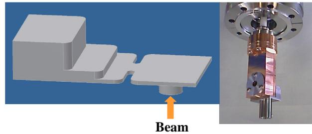
Figure 3: The output cavity of the test tube.
