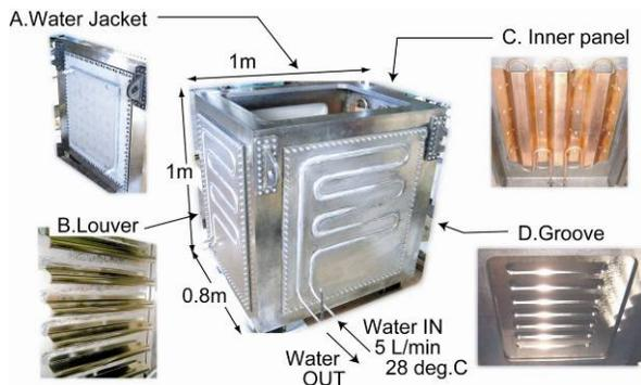
Figure 1: The model tank and the cooling panels.
