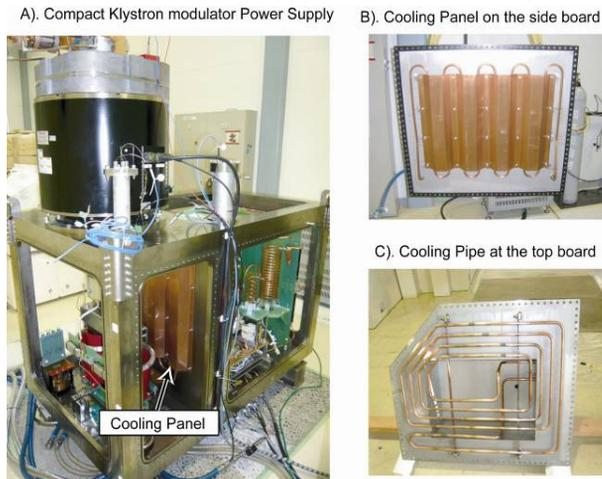
Figure 3: View of the compact klystron modulator, and the cooling system.
