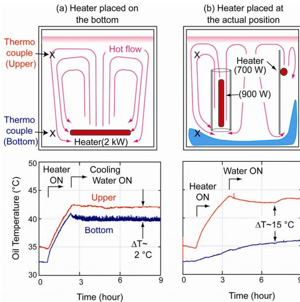
Figure 2: Upper figures show the schematic layouts of the experiments, and lower figures show the oil temperatures at the upper area and the bottom area of the model tank.
