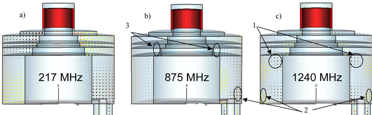
Figure 2: (a) H-Field distribution for the operating frequency 216,816MHz, (b) for the parasitic mode at 875MHz, and (c) for the parasitic mode at 1240MHz.
