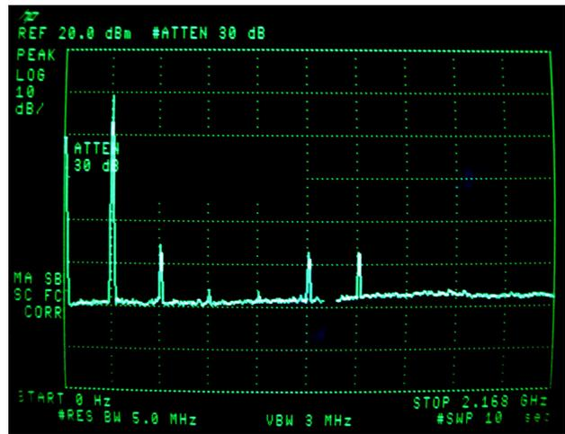
Figure 5: Measured spectrum with the new optimized ferrite setting.
