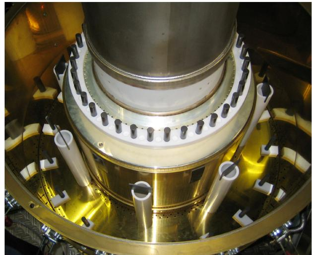
Figure 3: Ferrite arrangement as result of considerations based on the theoretical simulated H-field distribution.
