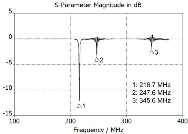
Figure 1: simulated  $|S_{11}|$  as function of frequency.
