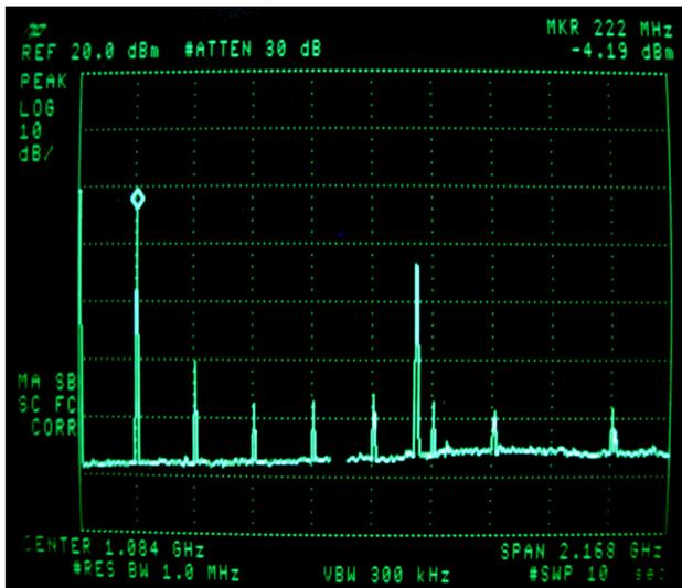
Figure 4: Measured spectrum with a coupling loop in the anode circuit with ferrites only in area 3.
