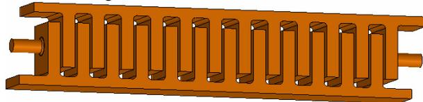
Figure 4: Example of a 24 cell, 15.75 cm zipper structure.
