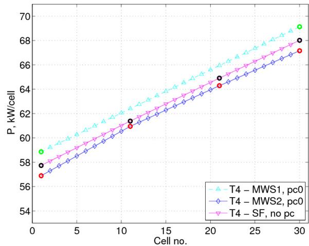
Figure 4: MWS and Superfish result interpolation for surface losses in the DTL tank 4.
