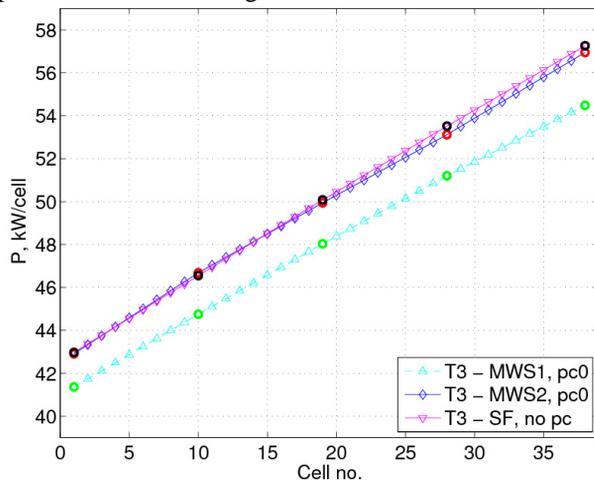
Figure 3: MWS and Superfish result interpolation for surface losses in the DTL tank 3.
