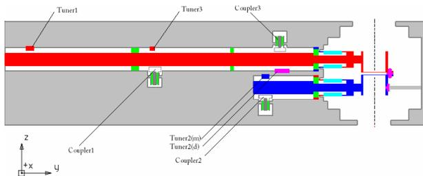
Figure 2: Layout of the triple harmonic buncher.
