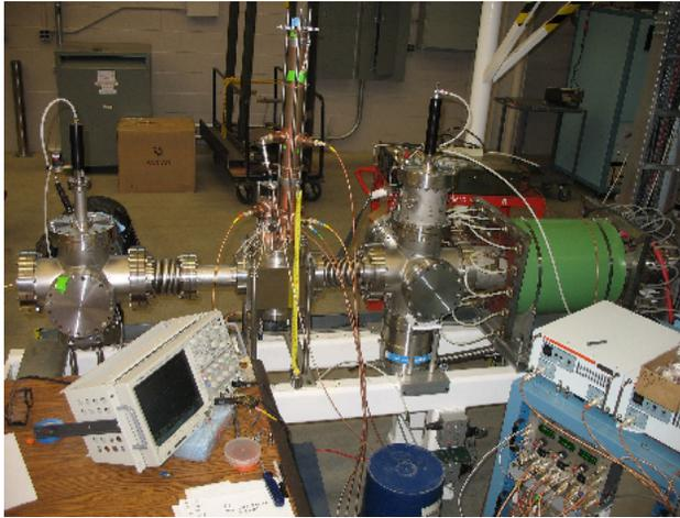
Figure 4: Experimental setup for the beam test of the triple harmonic buncher.
