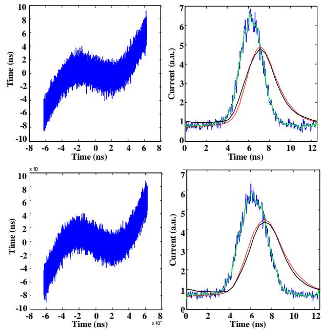
Figure 5: Temporal distributions at the entrance of buncher vs. at the FFC (left), projected temporal profiles (right): raw data (blue), smoothed data (green), trace from scope (black), fitted distribution (red), with initial beam energy spread  $\Delta E=11.5\text{eV/u}$  and FFC time response constant  $\tau=1.6\text{ns}$ . Buncher voltage  $V_b=174\text{V}$  (tops) and  $V_b=205\text{V}$  (bottoms).
