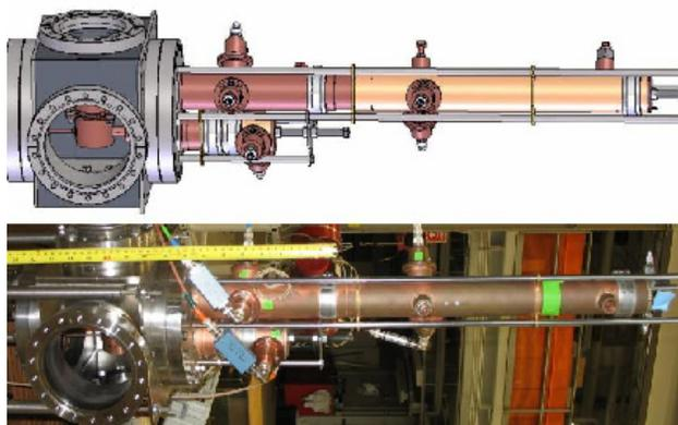
Figure 1: Triple harmonic buncher with two coaxial resonators and a single gridded gap: design drawing (top), photograph (bottom).
