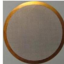
Figure 3: The 0.005" thickness and 50 mm diameter copper grid. Square mesh with grid width of 0.005" spaced 1mm apart.
