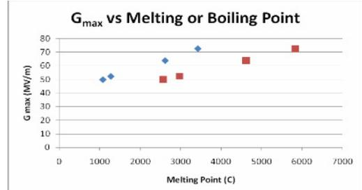
Figure 6: Maximum stable gradient as a function of metallic melting point (blue diamonds) or boiling point (red squares). From left to right, the four data points correspond to Cu, Be, Mo, and W.
