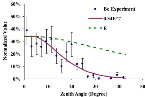
Figure 3: Be breakdown area fraction vs. zenith angle.
