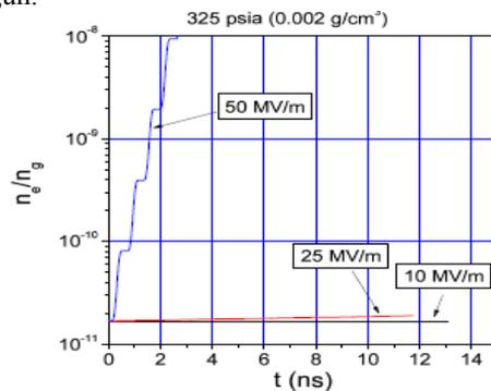
Figure 7: Electron density as a function of time at 805 MHz and gas density  $0.002 \text{ g/cm}^3$ .
