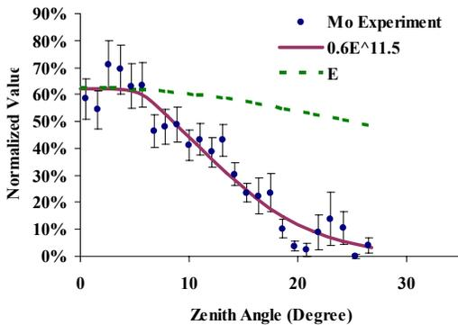
Figure 4: Mo breakdown area fraction vs. zenith angle.
