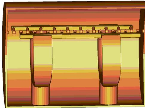
Figure 7: Long SR DT cavity with two supporting rings,  $N_p = 21$ .
