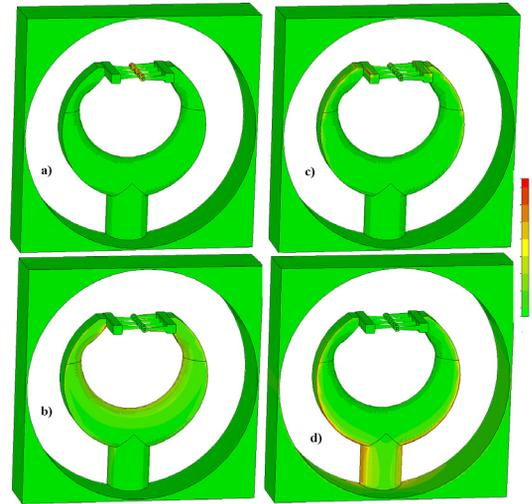
Figure 4: Electric  $\epsilon_0 E^2$  (a),(c) and magnetic  $\mu_0 H^2$  (b),(d) energy density distribution at the structure surface for operating (a),(b) and parasitic (c),(d) modes.
