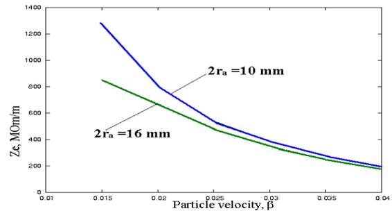
Figure 2:  $Z_e$  dependence on  $\beta$  for aperture diameters  $2r_a = 10mm$  and  $2r_a = 16mm$ ,  $\alpha = 0.5$ .
