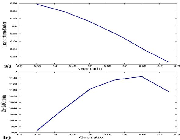
Figure 3:  $T(\alpha)$  and  $Z_e(\alpha)$  dependences for  $\beta = 0.015, 2r_a = 10mm$ .
