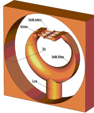
Figure 1: Proposed structure with Split Ring RF circuit and Drift Tubes. Half of the structure period.
