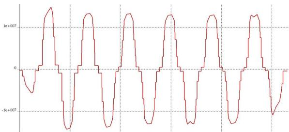
Figure 6: Electric field distribution along the beam axis in the short SR DT cavity.
