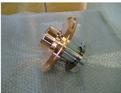
Figure 3: Three major components of the 216 MHz cavity. From left to right: short electrode with the end plate, inner conductor with the end plate, and the outer conductor.
