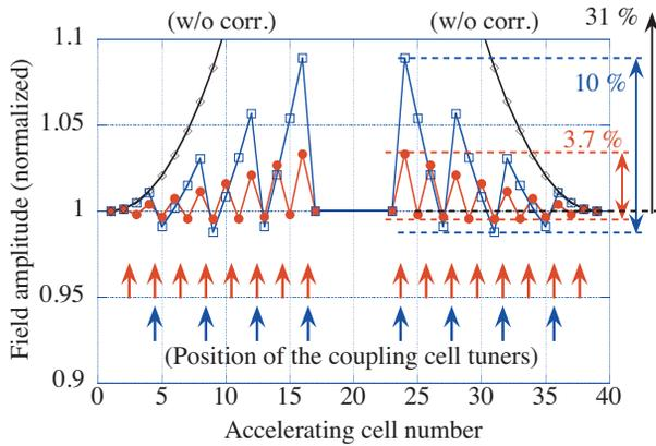
Figure 2: Simulated electric field distribution after the coupling mode frequency correction. The vertical axis is normalized at the first cell (#1). The arrows indicate the tuner position for the coupling cells. The red plot shows the case of the every two cells correction, the blue plot shows the every four cells correction, and the black plot shows the without correction.
