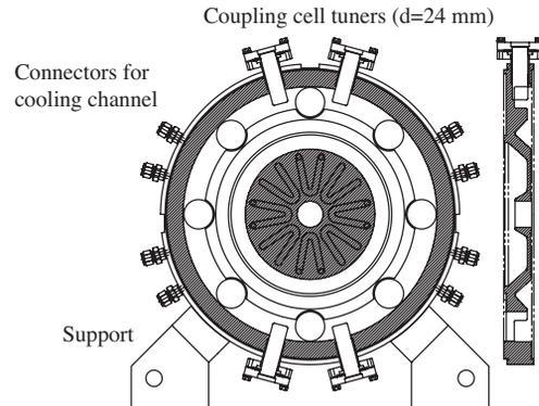
Figure 4: Draft design of the fixed coupling cell tuner. The four tuners are able to be attached for the maximum case.
