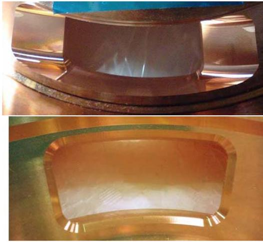
Figure 1: Simplified machining slots. The top is the coupling cell side view, the bottom is the accelerating cell side view.
