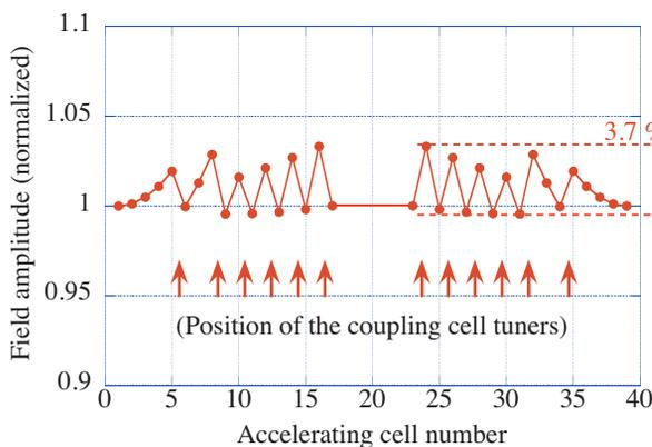
Figure 3: Simulated electric field distribution after the coupling mode frequency correction. The vertical axis is normalized at the first cell (#1). The arrows indicate the tuner position for the coupling cells. The total 12 coupling cells are corrected mainly around the center part of the module.
