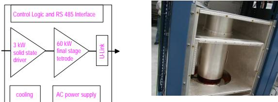
Figure 4: Scheme of the 60 kW amplifier and tube cavity.
