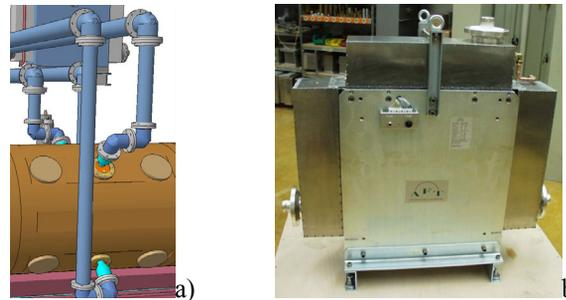
Figure 2: The four lines combined into the cavity and a 60 kW circulator.
