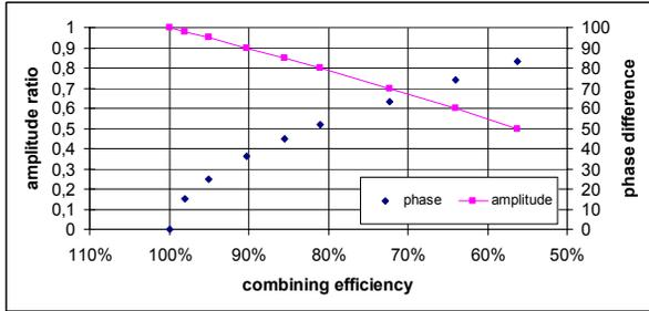
Figure 3: Effect of amplitude and phase difference in a 2-way combiner.
