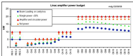
Figure 6: Requirements and choice of the linac amplifiers.
