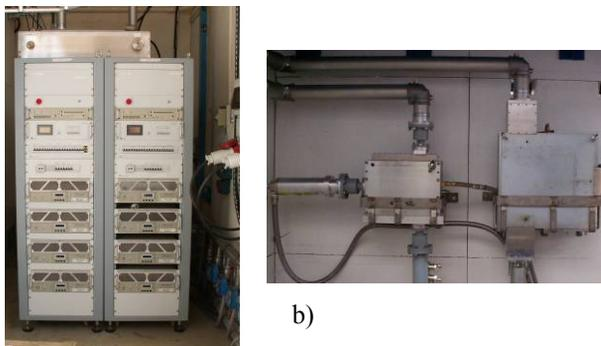
Figure 8 : Two 10 kW amplifiers installed at Orsay. Can be combined to obtain 20 kW. B) 10 and 20 kW circulators.
