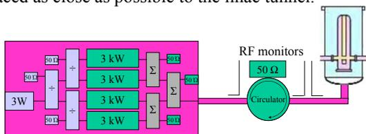
Figure 7 : Amplifier architecture. Circulators and dummy load are out of the amplifier cabinet, at the high power level. Green elements are water cooled.
