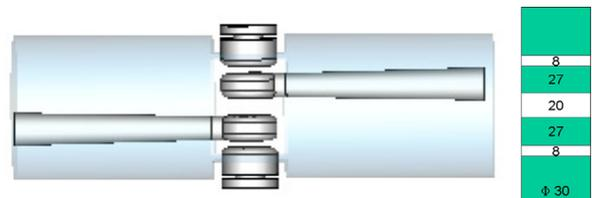
Figure 9: 176 MHz, beta 0.056 cavity and electrode geometry.
