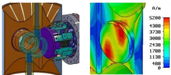
Figure 3: a) The tuner with flexible belts for RF and thermal contact; b) the current distribution.
