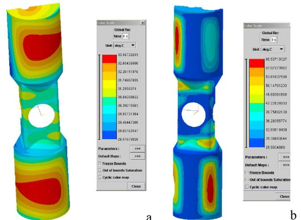
Figure 5: Temp. maps: a, solid copper, b: plated.
