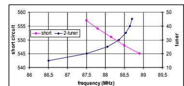
Figure 2: The RF structure. Tuner and shorting plate responses
