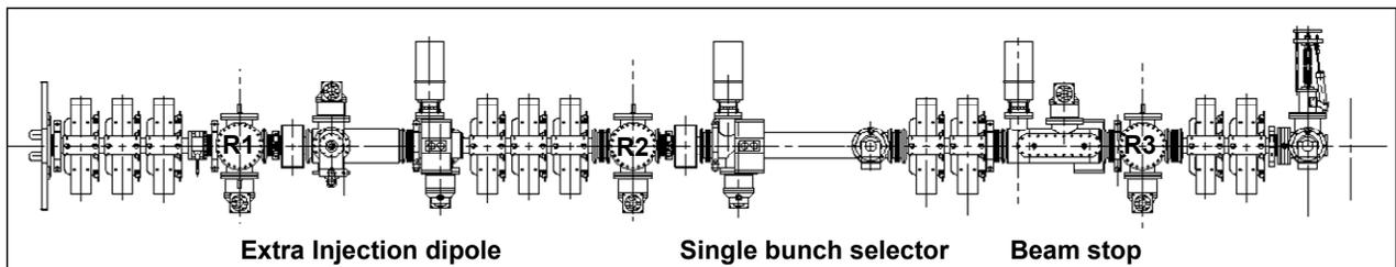
Figure 1: The medium energy beam transport line.
