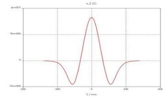
Electric field on the beam axis (@1 joule of stored energy)
