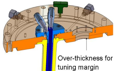
Figure 8: Stem cooling circuit and tuning margins.
