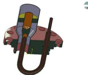
Figure 4: The coupling loop.
