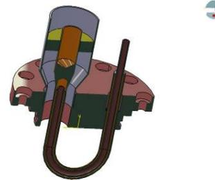
Figure 4: The coupling loop.
