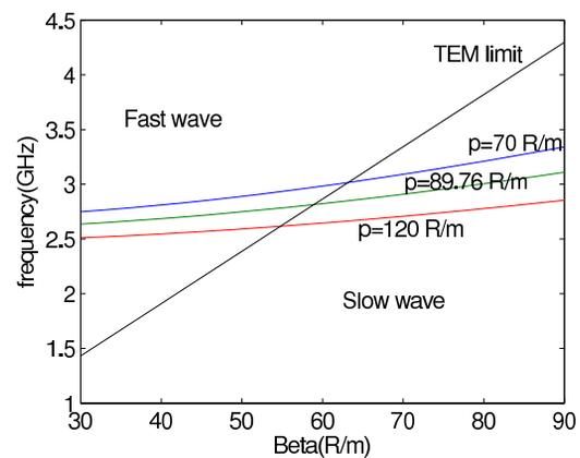
Figure 3: Dispersion diagram for twisted disk-loaded equivalent structure for several twist rates. (Twist rates in radians/meter.)
