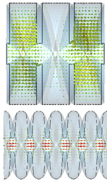
Figure 2: CST Simulation of Twisted disk loaded analog and SNS cavity analog: Electric field
