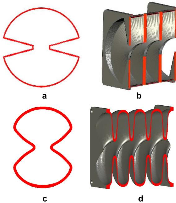
Figure 1: (a) “Notched” cross section of twisted disk-loaded analog. (b) 3D Cutaway view of twisted disk-loaded analog. (c) “Dumbbell” cross section of elliptical twisted analog. (d) 3D Cutaway view of elliptical twisted analog.
