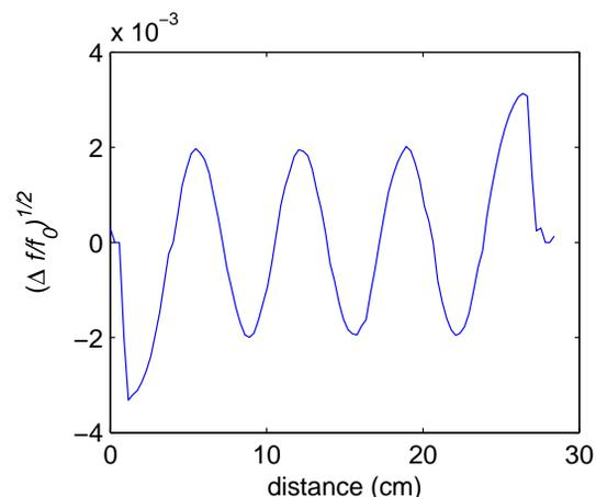
Figure 6: Measured (bead pull) results for elliptical twisted cavity prototype.
