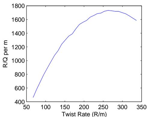
Figure 4: Simulated traveling wave  $\frac{R}{Q}$  as a function of twist rate in a twisted analog of a disk-loaded accelerating structure.
