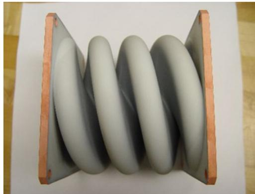
Figure 5: Prototype of a twisted elliptical cavity.
