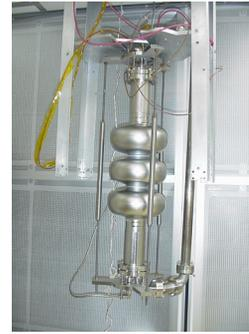
Figure 2: 3-cell cavity attached to test stand with external support rods. The cavity is located in the clean room in front of a horizontal laminar flow system.
