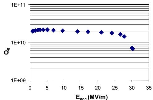
Figure 3: Performance of seamless 9-cell TESLA cavity.
