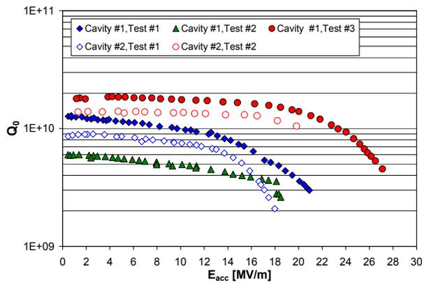
Figure 4: Summary of test results at 2 K from cavity 1 and 2. The total material removal was 150 $\mu\text{m}$  (test 1), 200 $\mu\text{m}$  (test 2) and 220  $\mu\text{m}$  (test 3) for cavity 1; 200 $\mu\text{m}$  (test 1) and 250 $\mu\text{m}$  (test 2) for cavity 2.
