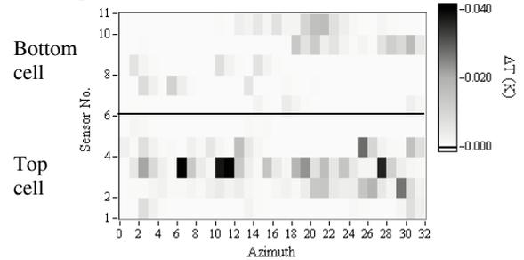
Figure 5: “Unfolded” T-map at the highest field achieved in cavity 1, test 3. The “azimuth” variable covers the cell’s circumference, while “sensor no.” covers a region  $\sim 4\text{ cm}$  on each side of the cells’ equator (on rows no. 3 and 8). Hot-spots are visible in the equator area of both cells.
