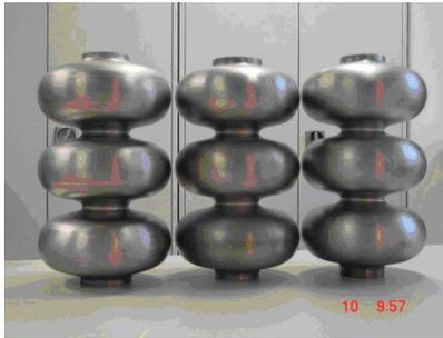
Figure 1: Hydroformed 3-cell niobium cavities.
