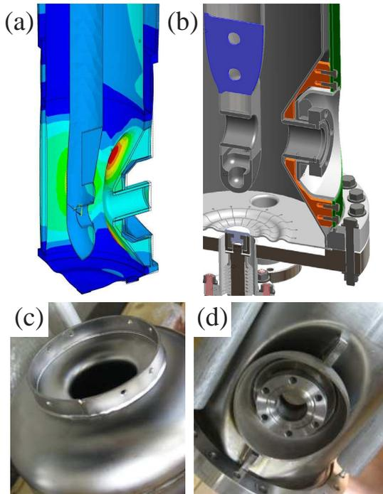
Figure 4: Stiffening of the  $\beta_m = 0.041$  QWR: (a) ANSYS model showing the predicted deformation for a stiffened QWR; (b) drawing of QWR with center conductor rib (blue) and beam port buttresses (orange); (c) Nb ring welded to the top of the cavity; (d) Nb buttresses welded to the beam port region.
