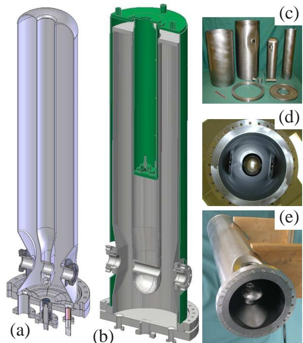
Figure 1: Drawings: (a) second generation  $\beta_m = 0.041$  QWR; (b) first generation  $\beta_m = 0.085$  QWR with damper and He vessel, shown in green. Photographs: (c) parts for first generation  $\beta_m = 0.085$  QWR and (d) completed cavity; (e) completed second generation  $\beta_m = 0.041$  QWR.
