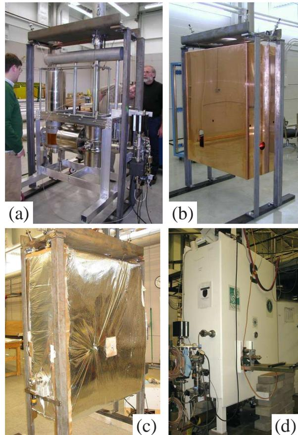
Figure 2: Construction of the low- $\beta$  test cryomodule: (a) cold mass hanging from top plate; (b) 77 K shield; (c) outer multi-layer insulation; (d) vacuum vessel.
