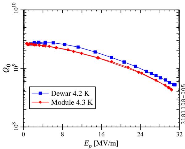
Figure 3: RF test results for the  $\beta_m = 0.085$  QWR: comparison of Dewar test and cryomodule test (after solenoid operation, temperature cycling, and He processing).
