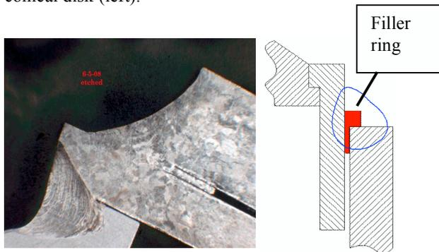
Figure 3: Drawing on the right shows titanium filler ring inserted in the gap between the spacer ring and the inner wall of the helium vessel shell. On the left is the TIG fillet weld sample generated using final weld parameters.
