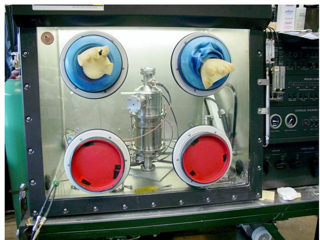
Figure 5: Glove box with cavity installed for TIG welding. Note the cables for monitoring the frequency spectrum of the cavity, and the lines for passing argon through the cavity and helium vessel during welding.
