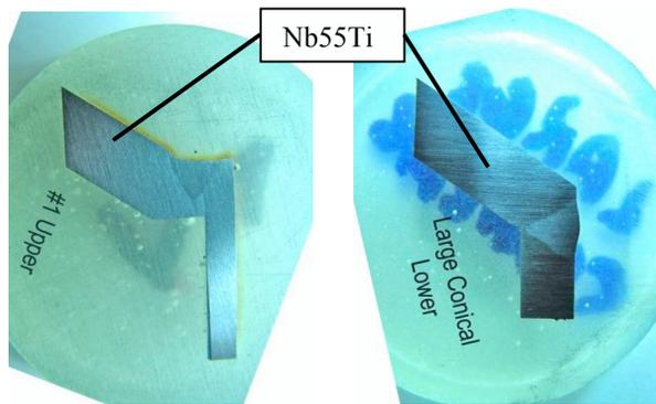
Figure 2: EB weld samples of helium vessel Ti shell to large conical disk (right), and Ti spacer ring to small conical disk (left).
