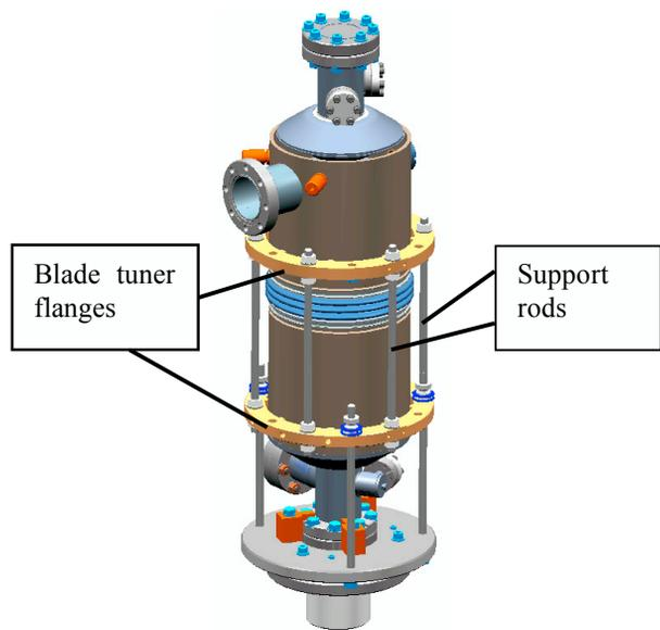
Figure 4: Cavity with helium vessel assembled in EB welding fixture.
