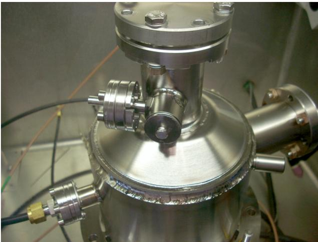
Figure 7: Close-up view of 3<sup>rd</sup> harmonic cavity with helium vessel after TIG welding is complete.
