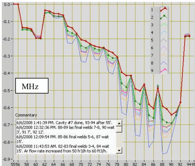
Figure 6: Frequency spectrum of cavity No. 7 recorded during TIG welding. The horizontal axis is time.
