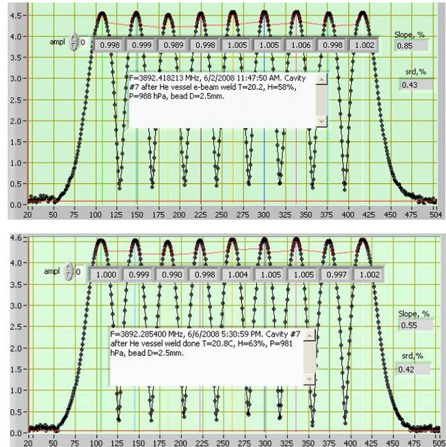
Figure 8: Field distribution of cavity No. 7 after EB welding and before TIG welding (top), and after TIG welding (bottom).
