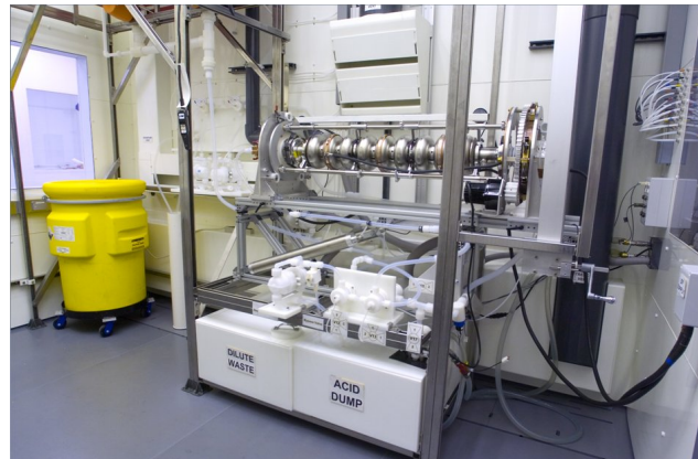
Figure 1: An electropolishing system for single- and multi-cell 1.3 GHz elliptical cavities at ANL
