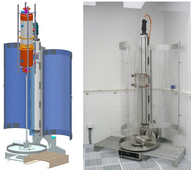
Figure 2: High-pressure rinsing system installed by Fermilab at the joint ANL/FNAL facility.
