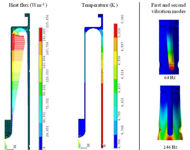
Figure 3: Heat flux input and resulting temperature distribution in the cavity, considering the thermal conductivity of copper RRR=100 and 4.5 K He I pool boiling cooling in convection and nucleate boiling regimes. First and second vibration mode shapes and corresponding frequencies.
