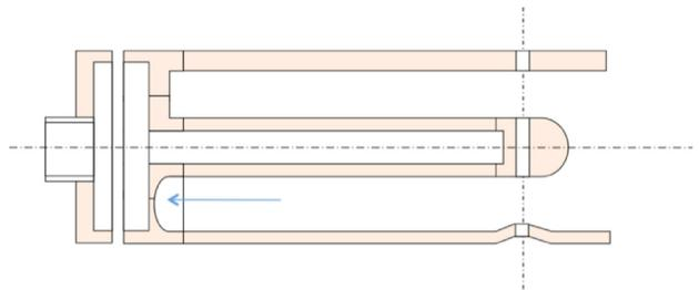
Figure 4: Manufacturing sequence of the cavity. The top half of the drawing illustrates the shape of the raw pieces, the bottom one the final shape. The arrow indicates the region of the final circular long-throw welding.
