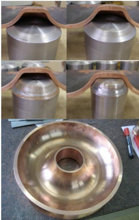
Figure 5: Sequence of the different drawing steps leading to the final form for the beam ports, and full scale test piece for the long-throw e-beam welding.
