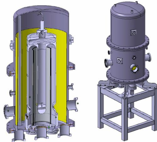
Figure 6: 3D views of the coating system.
