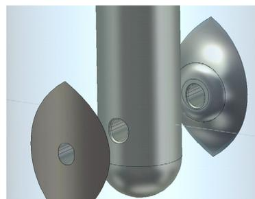
Figure 2: Details of beam port.
