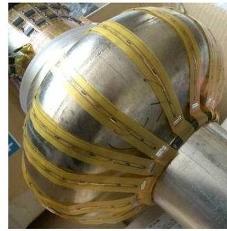
Figure 10: The flexible PCB
