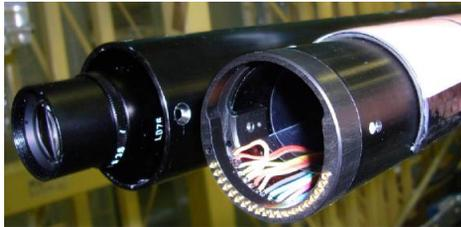
Figure 5: The camera and new head assembly. They can be easily separated and all the electrical connections are through the pins, which makes the assemblage and maintenance easy. Left: Camera cylinder. Right: Head assembly.
