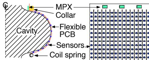
Figure 9: Conceptual sketch of an easy installation of sensors. The sensors are mounted on a flexible PCB that is wrapped around the cavity cell.
