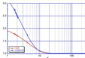
Figure 8: Measured resistances of 1kΩ and 10kΩ chip resistors as a function of temperature. The fitting curves are just guides for eyes.
