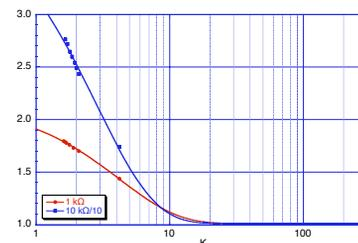
Figure 8: Measured resistances of 1kΩ and 10kΩ chip resistors as a function of temperature. The fitting curves are just guides for eyes.
