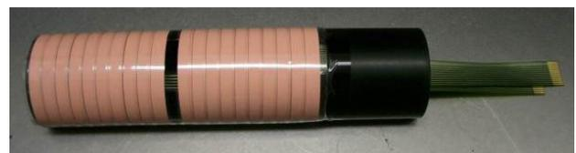
Figure 3: New EL stripe illuminator. The strip width is reduced from 10 mm to 7 mm; hence, the number of strips increases from 14 to 20. The camera looks through a peephole located at the center of strips.
