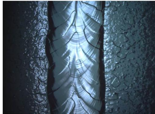
Figure 7: The inner surface (EBW seam) of SC cavity before (top) and after EP process (bottom, 125 μm removed.). The picture size is 13 mm x 9 mm.
