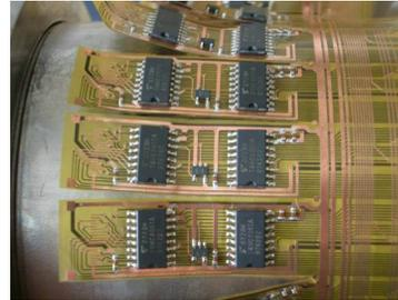
Figure 11: Analog multiplexers mounted on a demonstration setup.
