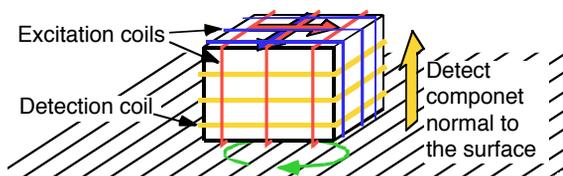
Figure 13: Excitation coil configuration. They generate a rotating magnetic field on the specimen surface.
