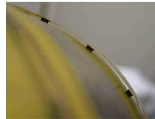
Figure 12: Sensors mounted on a flexible PCB are pushed against the wall surface.
