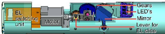
Figure 4: The new head assembly. The mirror is tilted by the pulse motor to change the sight line. Coaxially illuminating LED's located before the mirror enable us to observe a surface normal to the sight line of the camera at any mirror angle, where the EL strip is absent for the peephole. The EL sheet slides with the mirror angle by a lever to keep the peephole on the sight line.
