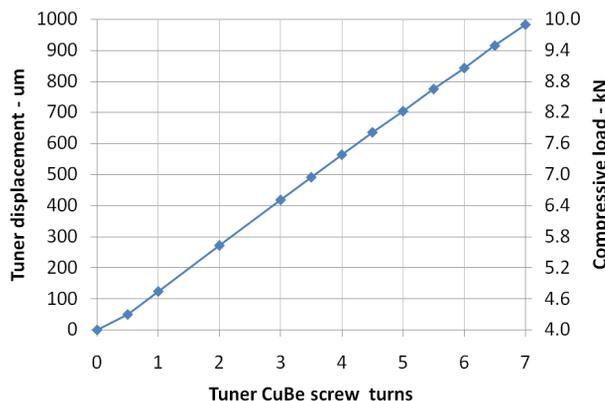
Figure 6: Compressive load test on ILCTA tuner
