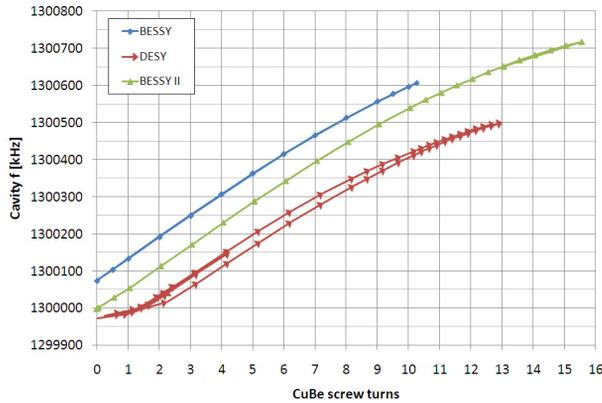
Figure 2: Tuning range tests in CHECHIA and HoBiCaT.
