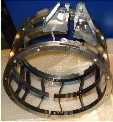
Figure 4: One of the Blade Tuner manufactured for ILCTA\_NML facility at Fermilab.
