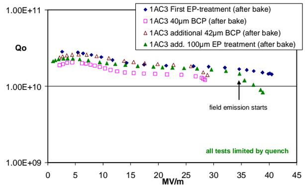
Figure 2: Q(E)-performance of an EP - BCP - BCP - EP preparation cycle of single-cell cavity 1AC3.
