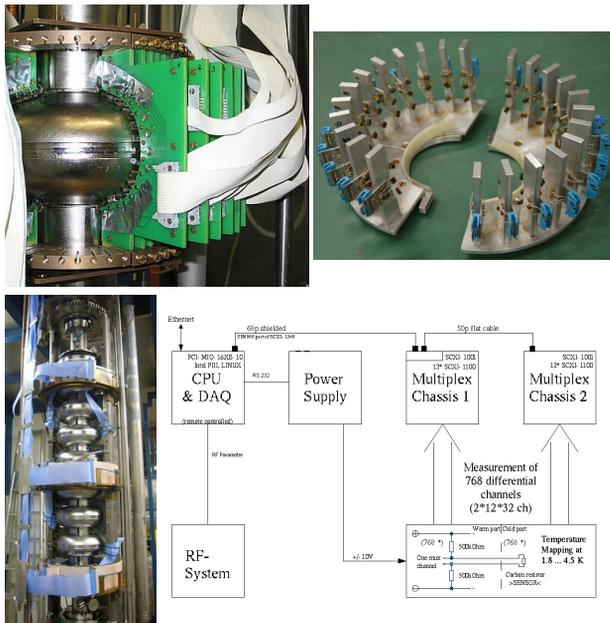
Figure 1: a) Single-cell T-map system (top left); b) rotating nine-cell T-map system (bottom left); c) “quick fixed” T-map (top right); d) data acquisition scheme (bottom right).
