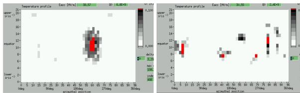
Figure 5: (left) Quench at 39 MV/m in single-cell 1AC4, test 6; (right): after  $41 \mu\text{m}$  BCP a “hot spot” is visible at identical location in test 7, 1AC4.
