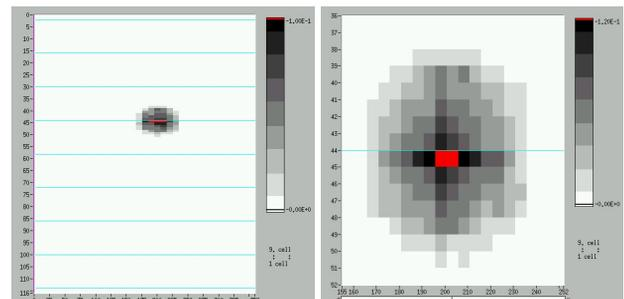
Figure 3: Identification of quench location at equator in cell 6 of nine-cell Z111 at 16 MV/m; left: Full rotating T-Map; right: Cell 6 with refined angle resolution.
