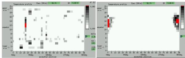
Figure 4: (left): Just below the quench field at 39 MV/m: typical field emission trace and heating at iris visible; (right): Quench at 39 MV/m located close above the equator (both T-maps taken in test 7 of single-cell 1AC3).
