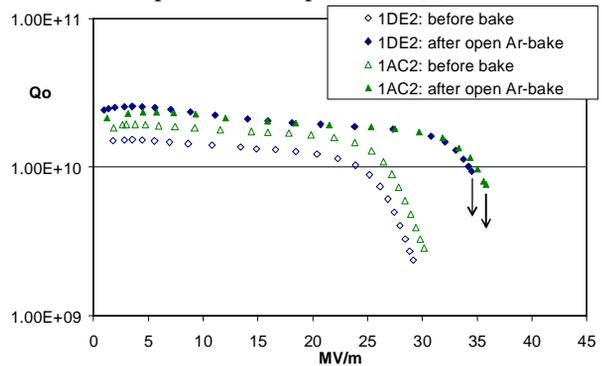
Figure 4: Effect of open Ar-bake after final short BCP on two single-cell cavities fabricated of fine-grain Nb.
