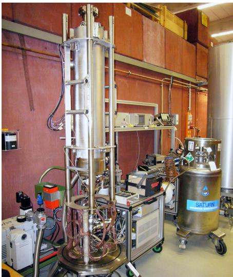
Figure 1: DESY bake stand for UHV bake.
