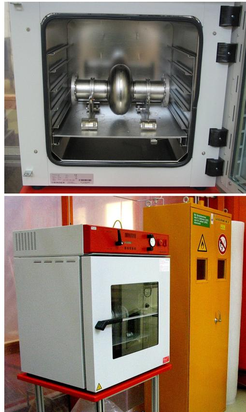
Figure 2: Vacuum drying cabinet for single-cell cavities.
