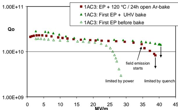
Figure 3: Effect of open Ar-bake and UHV-bake on an electropolished single-cell cavity made of large grain niobium (1AC3).
