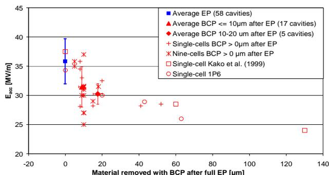
Figure 5: Cavity data for cavities with etching after electropolishing. Data includes both single- and nine-cell results as well as fine- and large-grain niobium material. For comparison older KEK data [4] is also shown. Cavities with field emission limitation and fabrication defects are excluded.
