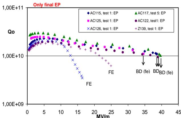
Figure 2 a): Vertical test results of most recent cavity production after EP as a final surface treatment. Strong field emission (FE) has been in two cavities causing a strong degradation of the quality factor. In two other cavities much smaller levels of radiation have been observed causing no significant degradation.
