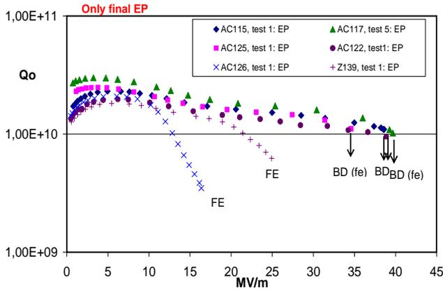
Figure 2 a): Vertical test results of most recent cavity production after EP as a final surface treatment. Strong field emission (FE) has been in two cavities causing a strong degradation of the quality factor. In two other cavities much smaller levels of radiation have been observed causing no significant degradation.
