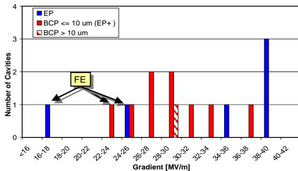
Figure 3: Comparison of the vertical test results for the final surface treatments.
