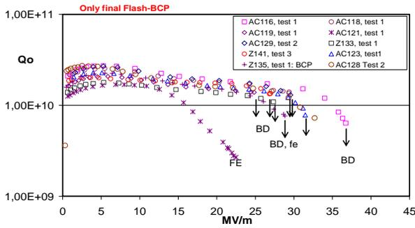
Figure 2 b): Vertical test results of most recent cavity production after etching (BCP=Buffered chemical polish) as a final surface treatment. One cavity shows strong FE.
