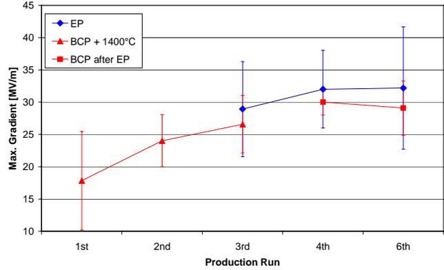
Figure 4: Comparison of final surface treatments for the cavity production runs at DESY. For comparison the maximum gradient in the last test of each cavity is shown. Note that data set for EP in 6th production is only six cavities so far. Re-tests of cavities with additional treatment have not yet been done. Other data sets include typically 10 – 20 cavities.
