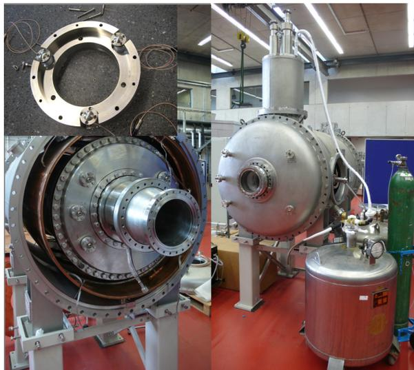
Figure 3: Horizontal cryostat with piezo tuner.
