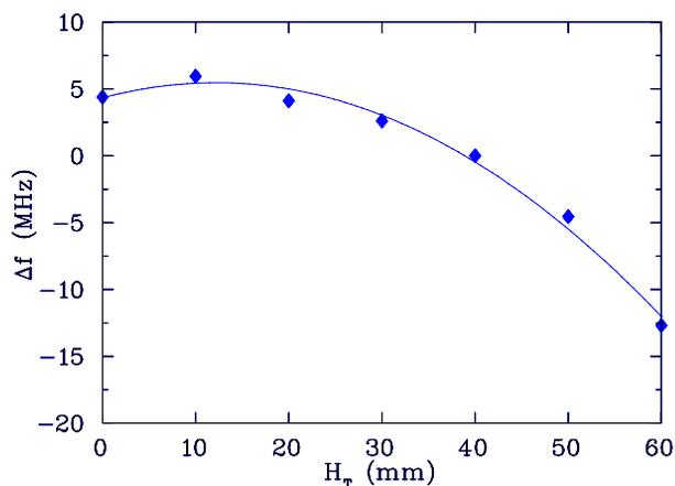
Figure 5: Frequency shift as function of the tuner height using all tuners simultaneously.
