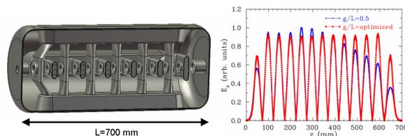
Figure 8: Geometry of the first superconducting CH-cavity for EUROTRANS (left) and the field distribution (right).
