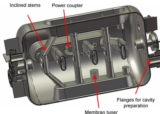
Figure 4: Geometry of the new superconducting 325 MHz CH-cavity.
