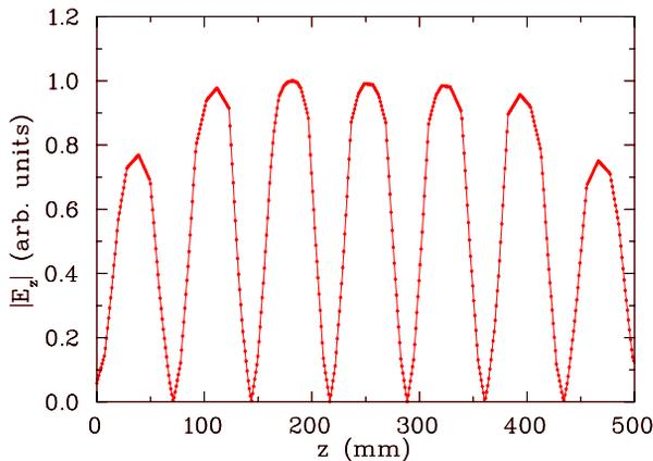
Figure 6: Simulated electric field distribution of the 325 MHz CH-cavity.
