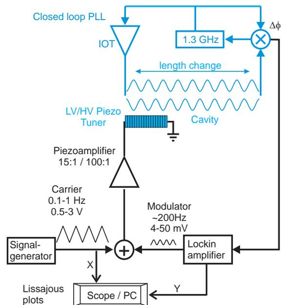
Figure 2: Experimental setup of the hysteresis measurements.
