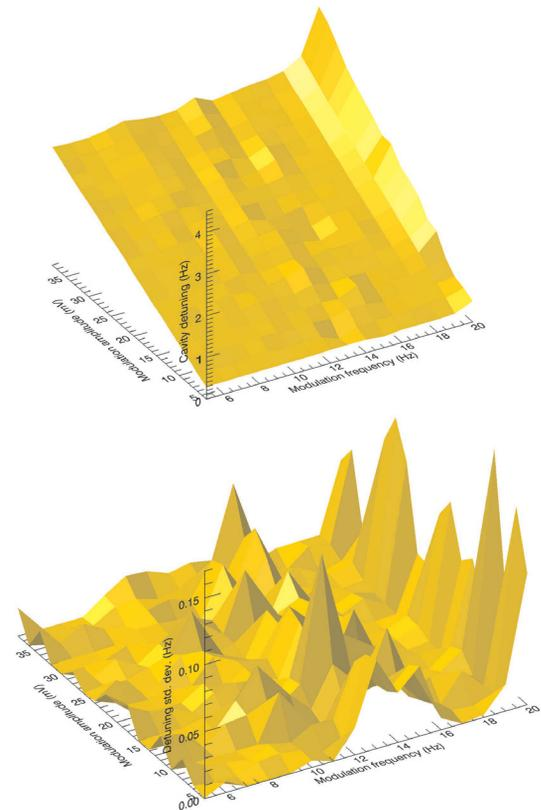
Figure 4: Measurement of piezo resolution without carrier (blade tuner, LV piezos). Upper picture: Low-frequency transfer function with amplitude scan. Lower picture: Standard deviation of the same measurement yielding estimates for the achievable piezo resolution. The measurement is overlapped by (very small scale) microphonics at 14 Hz and 20 Hz.
