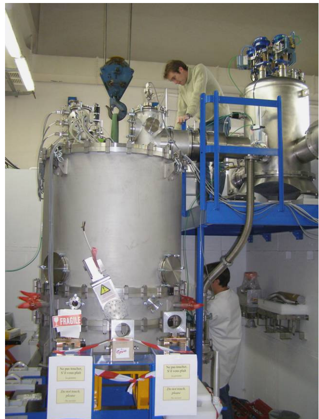
Figure 1: Spiral 2 cryomodule test stand at IPN Orsay.
