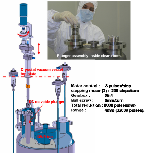
Figure 3: CTS with SC plunger insertion.
