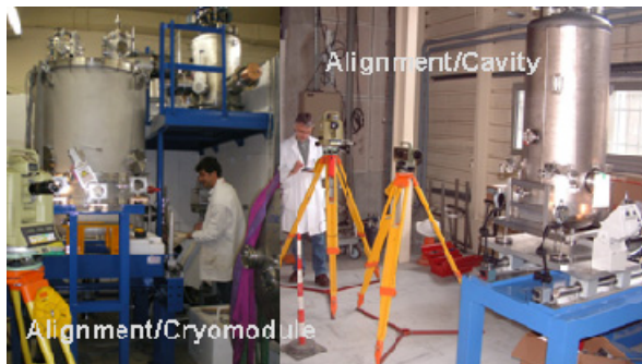
Figure 2: Cavity and cryomodule alignment.
