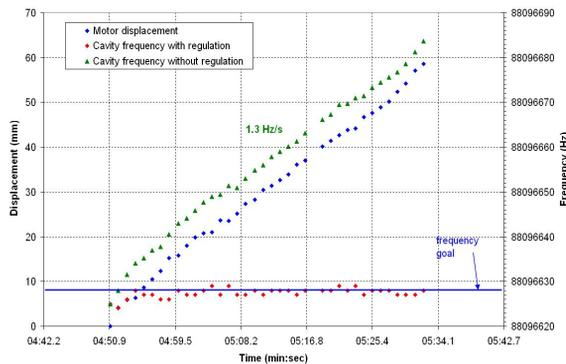
Figure 7: Slow frequency regulation test.
