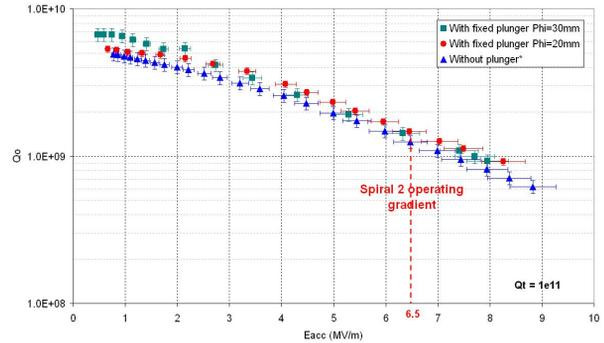
Figure 8: Q<sub>0</sub> versus accelerating field with  $\Phi = 30$ mm and 20mm plungers and without plunger.
