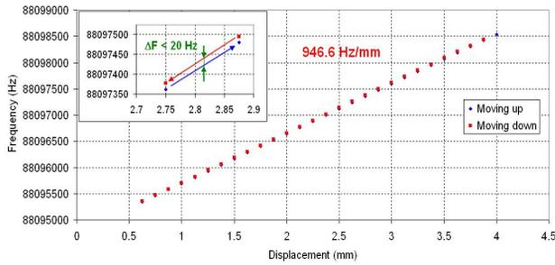
Figure 6: Frequency shift versus plunger. In the upper left corner, mechanical hysteresis when moving up and down.
