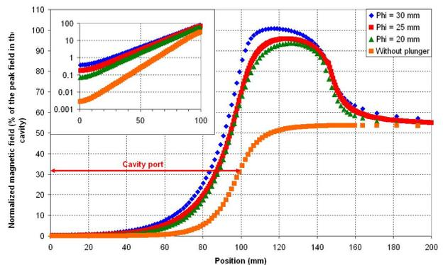
Figure 5: Magnetic field distribution along the plunger for different diameters.
