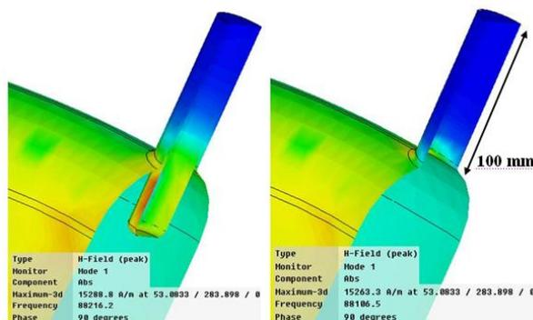
Figure 4: H-field distribution with and without the plunger.
