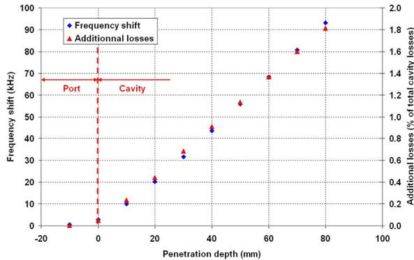
Figure 3: Frequency shift and additional losses versus penetration depth.
