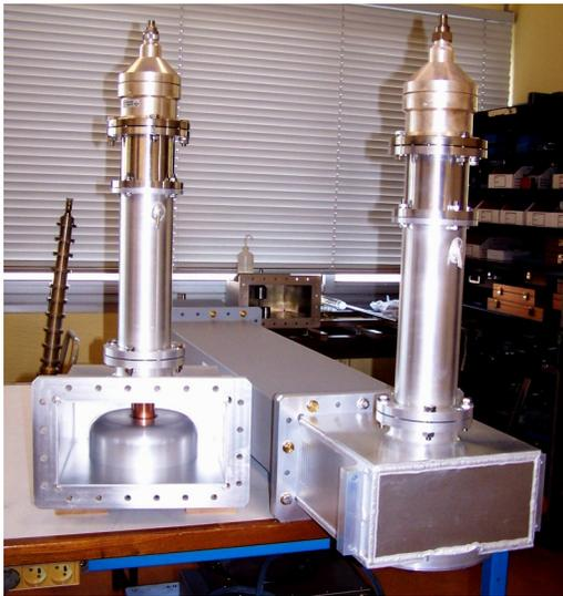
Figure 7: Doorknobs with adaptors for RF measurements.
