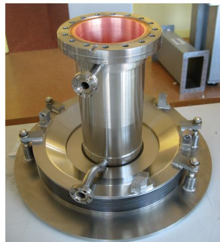
Figure 6: He cooled outer conductor.
