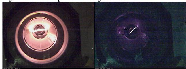
Figure 5: CCD camera views of a tungsten wire before sublimation (on the left) and during its breaking (right).
