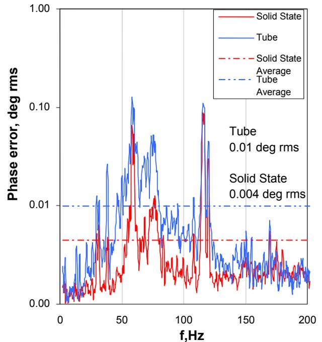
Figure 6: Phase noise measurements with the superconducting cavity
