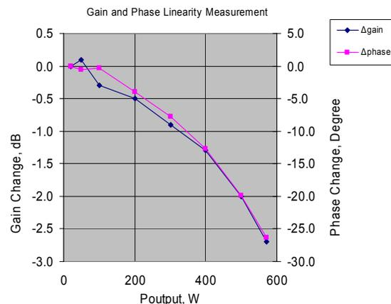
Figure 1: Gain and phase linearity measurement
