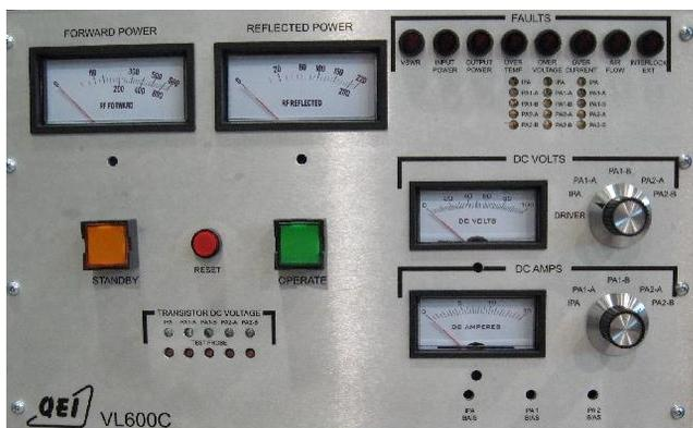
Figure 2. Photo of the front panel of the amplifier
