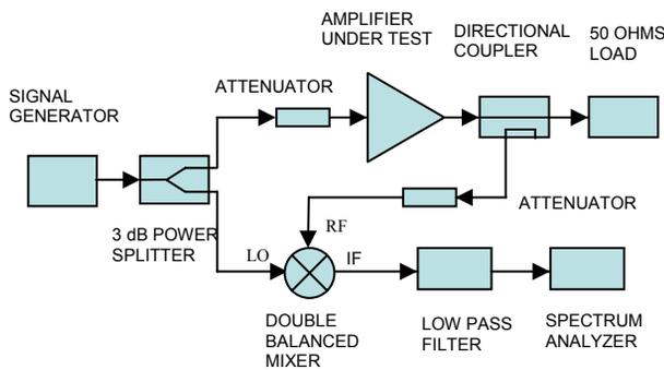
Figure 3: Basic block diagram of phase noise measurement
