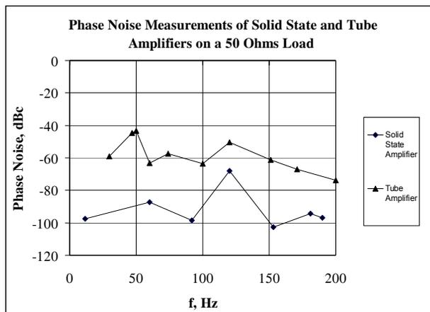
Figure 4: Phase noise measurement with a 50 ohms dummy load
