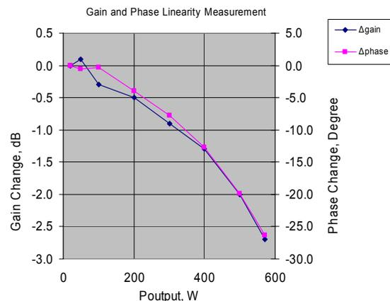
Figure 1: Gain and phase linearity measurement
