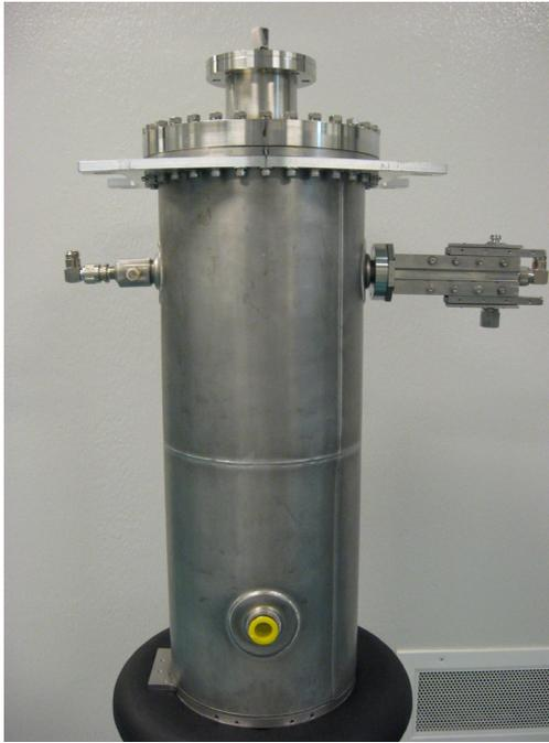
Figure 5: Photo of 141 MHz superconducting cavity used for the test
