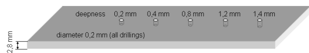
Figure 4: Schematic sketch of the test body for assessment of detection limit for volumetric defects (sheet thickness 2.8 mm).
