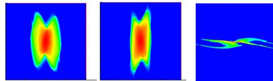
Figure 10: Phase space plots after 30 cells in the FNAL-PD RFQ. Left (x,x'), middle (y,y') and right (Δφ,ΔW/W).
