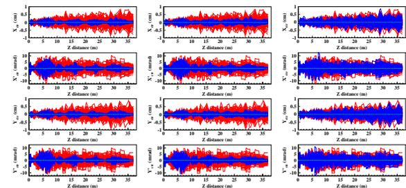
Figure 5: Effect of monitors precision on the correction: left: 10 $\mu$ , middle: 30 $\mu$  and right: 100 $\mu$ .
