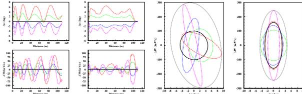
Figure 2: The left 4 plots show the phase and energy oscillations of the five charge states around the central charge state before and after applying the tuning procedure. The right 2 plots show the corresponding beam ellipses on the stripper before and after tuning.
