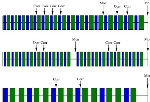
Figure 3: Monitors and correctors required for the front-end of the FNAL-PD linac.
