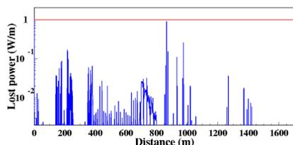
Figure 12: Beam loss in Watts/m in the FNAL-PD linac and transfer line. In red is the conventional 1 W/m limit.
