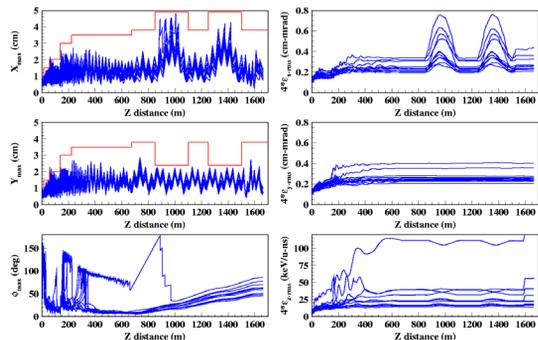
Figure 11: Beam envelopes (left) and emittances (right) along the FNAL-PD linac and transfer line for multiple seeds.
