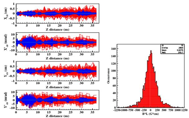
Figure 4: results of the correction procedure. On the right are beam centers in  $(x, x', y, y')$  before (red) and after (blue) correction. On the left is a distribution of required corrector strengths.
