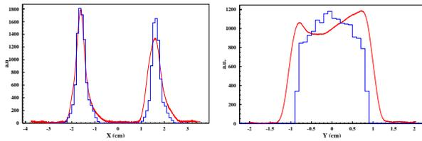
Figure 6: Horizontal (left) and vertical (right) beam profiles. The curves are the measured profiles and the histograms are the result of the TRACK fit.
