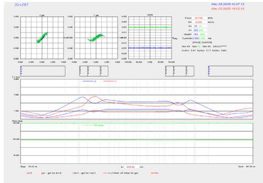
Figure 7: Result of a symmetric fit between the two LEBT magnets to recombine the two charge state Bi beams.
