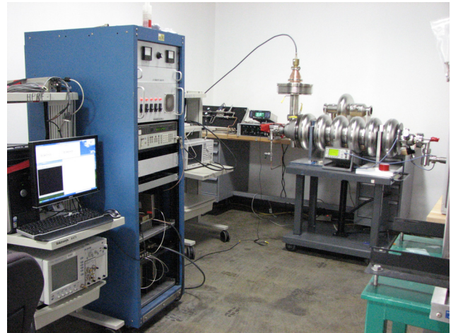
Figure 1: Plasma processing setup with HB Cavity.
