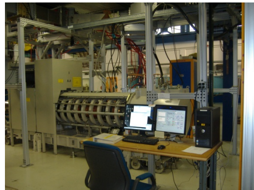
Figure 1: HINS Console and Klystron.
