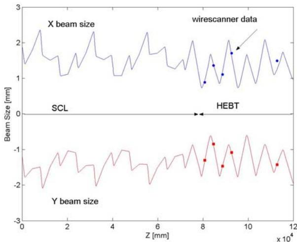
Figure 4: Plots of beam profiles after matching SCL to HEBT. Solid lines are plots of beam size  $\sigma$  [mm] from the Trace3D program and solid circles are wire-scanner measurement data.
