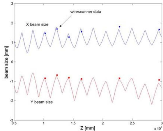
Figure 1: Plots of beam profiles before matching DTL to CCL. Solid lines are plots of beam size  $\sigma$  [mm] from the Trace3D program and solid circles are wire-scanner profile data. The peak beam current is 40 mA.
