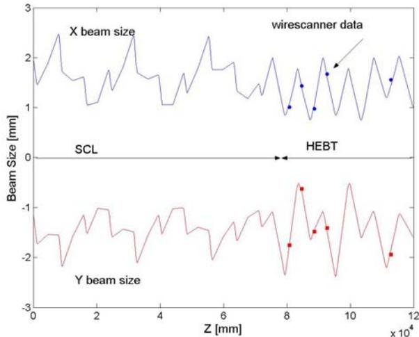
Figure 3: Plots of beam profiles before matching SCL to HEBT. Solid lines are plots of beam size  $\sigma$  [mm] from the Trace3D program and solid circles are wire-scanner measurement data.
